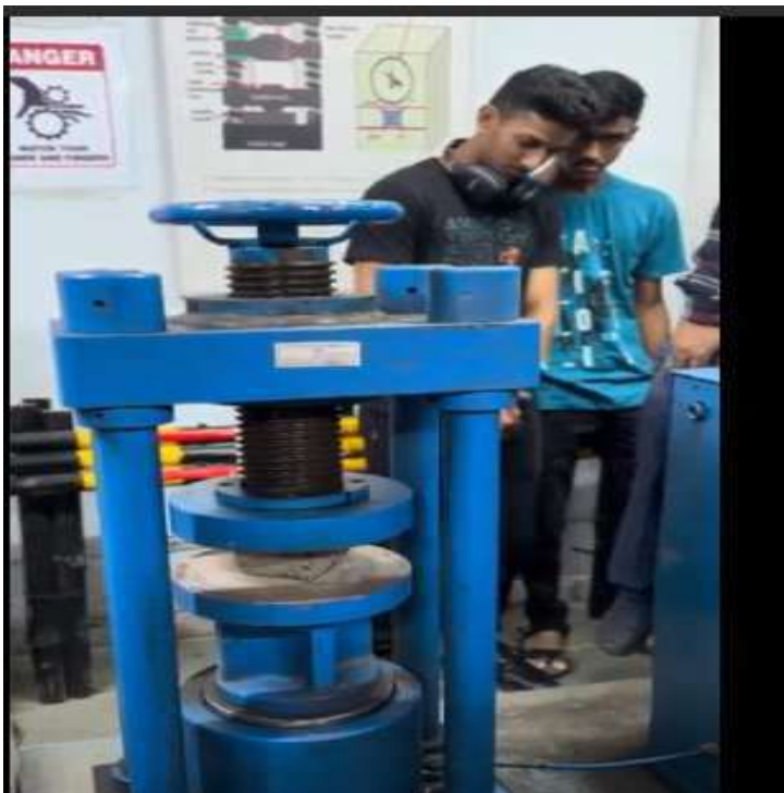
Fig :-CTM:-Concrete cube test
